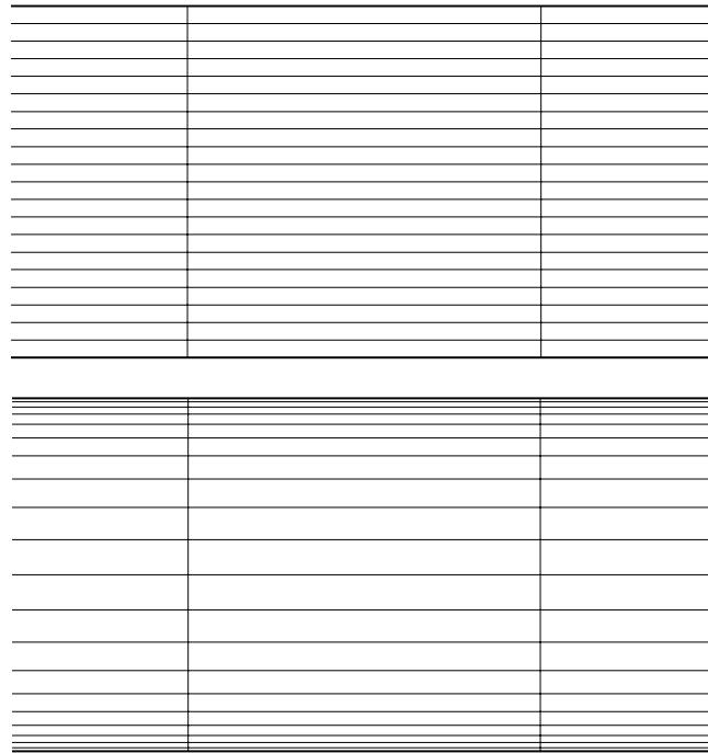
Fig. 2. The two mesh systems employed for evaluating the wall function and low Reynolds number treatments. The upper mesh is uniform in the transverse direction, and the lower mesh is non-uniform with the nearest wall cell assuming h/dy_1 = 100 , where dy_1 is height of the first cell adjacent to the wall.
